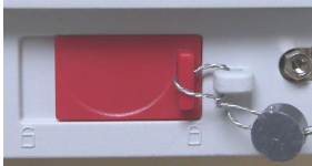
Locked with Wire Seal
